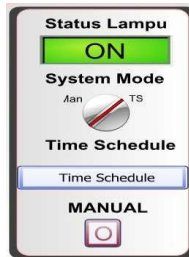
Figure 17 Auto selector monitoring graph (Time Schedule) Condition Lights On
