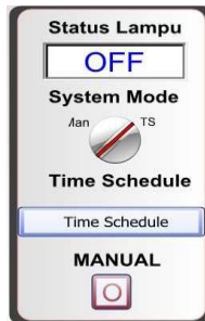
Figure 18 Monitoring graph for auto selector (Time Schedule) when the light is off
