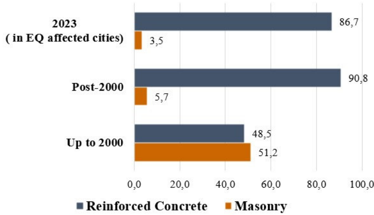
Figure 2. Time-based shifts in structural system types in Türkiye and eq. affected cities 1
